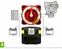
the starting and house circuits. For the house circuit, one terminal of a pair is connected to your accessories and the other to the positive terminal of your battery. On the starting circuit, one terminal is connected to your engine's wiring harness and the other to the positive terminal of the starting battery.
