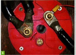
Both of the old battery switches were cracked (1), so Sheppard replaced them with a single **Dual Circuit Plus** and an Automatic **Charging Relay from** Blue Sea Systems (2). Sheppard altered things slightly, but the wiring diagram (3) is a good guide for how to hook things up.
