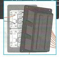
INSTALL THE PANEL Before securing the panel, energize each switch to ensure proper operation. Then remove the top and bottom cover plates and use the supplied self-tapping screws to mount the panel. Recheck the switches. To guard against short circuits, install a Blue Sea panel back cover on the rear of the distribution panel with four small self-tapping screws. Use the supplied adhesive labels to designate switch functions.
