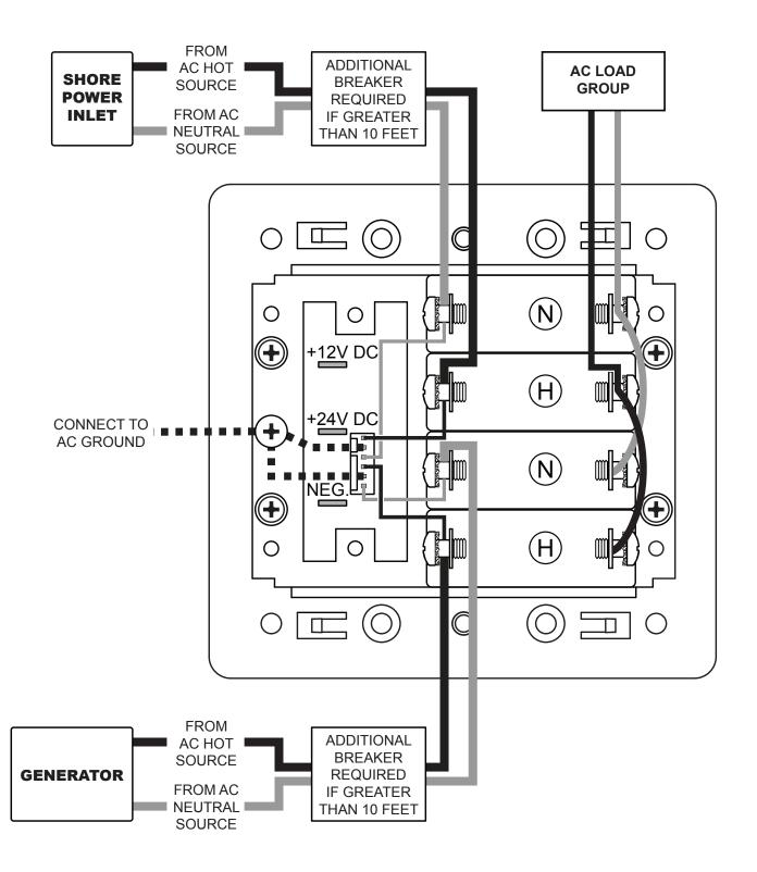
Panel Wiring Schematic AC Source Selection Panel
