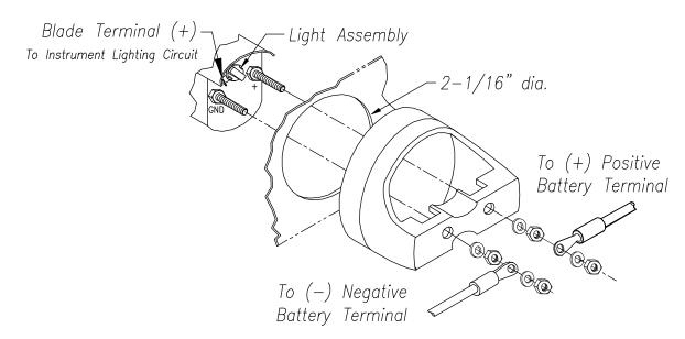
**<u>INTRODUCTION</u>**: The *Faria®* Battery Condition Indicator (BCI) is designed to display the relative state-of-charge of your 12V battery. The BCI monitors the battery voltage with a very high degree of resolution and accuracy according to the following chart:
